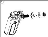
Remove the hex nut and nut collar from fill valve .Don't remove the seal !!!
