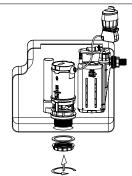
Insert the flush valve's base into the water tank. Screw on the nut collar and nut properly.
