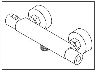
Screw your bar valve onto the easy fix kits. Water test again.
