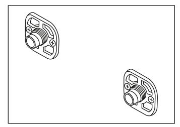
Place the olives onto the pipes, ensure olives are straight as the olives will bend when the main body is tightened to the backplate if inproperly placed.
