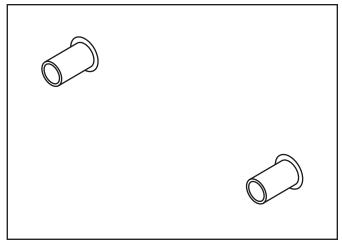
Cut the pipes down leaving 23mm protruding from the face of the wall. Do not leave any sharp edges or burrs on the pipes.
