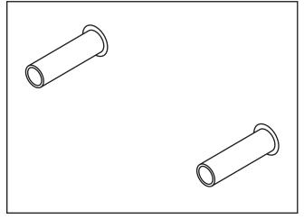
Ensure that your pipe centres are correct for your bar valve (usually 150mm) and ensure that your tiles / wall coverings are fully sealed and cured
