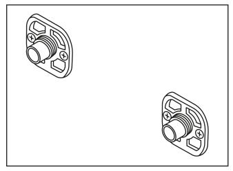
Place the backing plate over the pipe. Drill and screw the backing plate to the wall using a suitable method for your wall. Check for pipes and cables before drilling.
