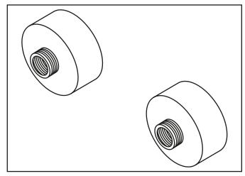
Screw your shrouds onto the main body, back to the wall. (Shroud not included)
