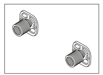
Screw the main body onto the backing plate, using an adjustable spanner to tighten. This will compress the olive and create a seal. You can now water test.
