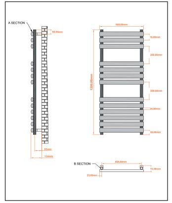
Dimensions (measurements in mm)
