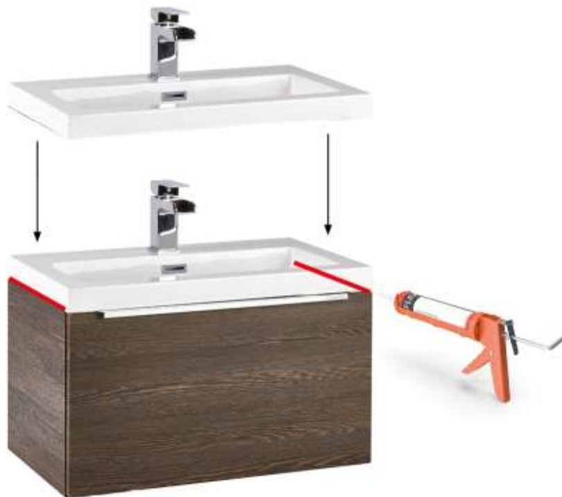
Silicone on top edge of the side panels only and lower basin on top of silicone to form a watertight seal
