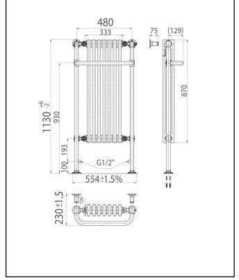
Dimensions (Measurements in mm)
