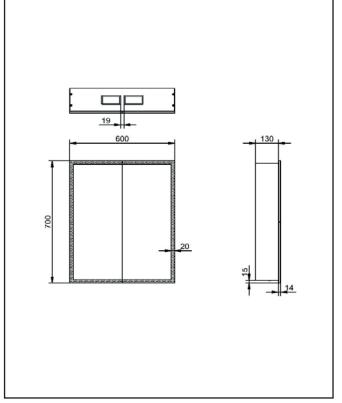
Dimensions (measurements in mm)
