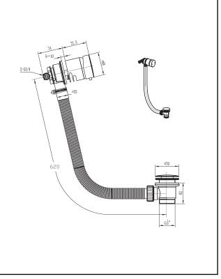
Dimensions (Measurements in mm)
